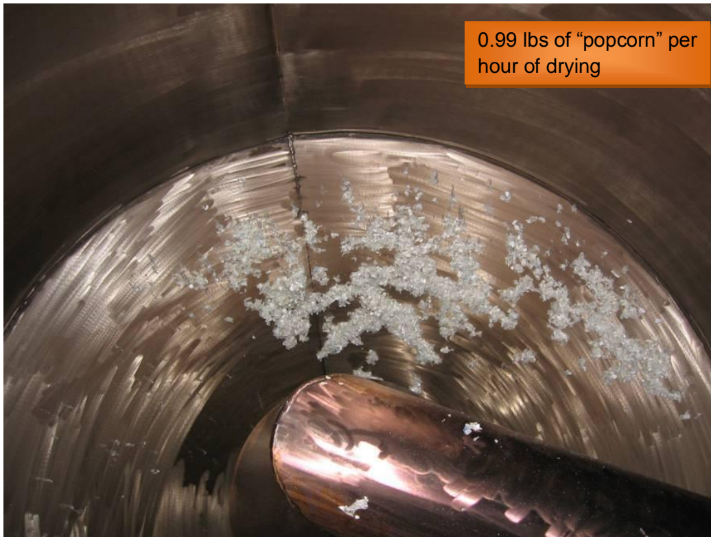
Figure 10 - PCR Flake w/1% PETG Inside of Dryer Cone after Testing
